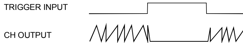
Fig. 2: Trigger input as gate signal
